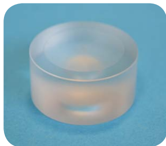
Powder/Thin film sample holder Material: PMMA Cavity: Diameter: 22 mm Depth: 0.2/0.5/1 mm
