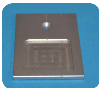
Front loading sample holder Material: Al Cavity: HxL: 20 mm x 20 mm Depth: 1 mm
