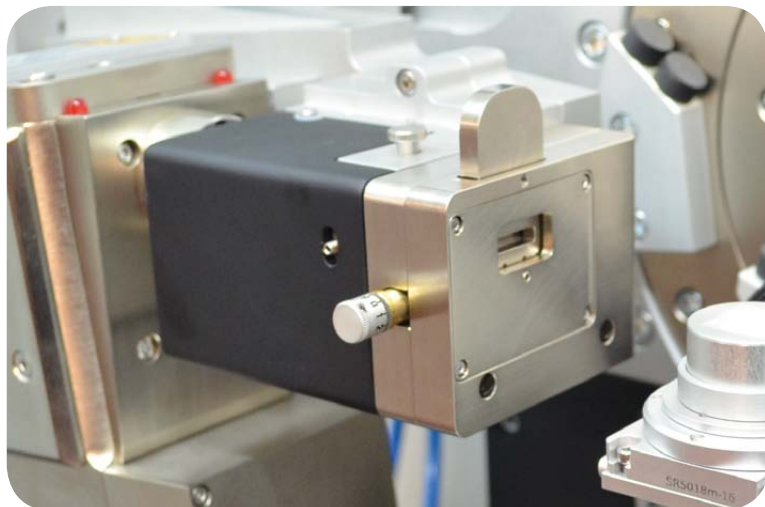
Parabolic mirror monochromator
