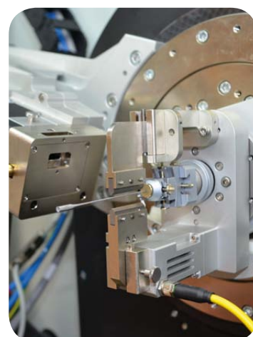
Capillary sample holder
