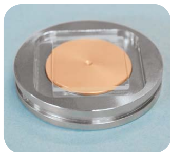
Clay oriented aggregate mount sample holder Material: steel and glass Cavity: Area: 37 x 37 mm 2 Depth: 2.5 mm Glass: 25x25 mm 2
