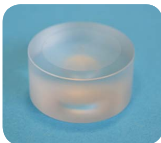
Powder/Thin film sample holder Material: PMMA Cavity: Diameter: 22 mm Depth: 0.2/0.5/1 mm
