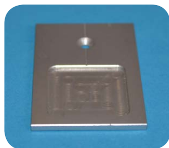
Front loading sample holder Material: Al Cavity: HxL: 20 mm x 20 mm Depth: 1 mm
