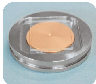
Clay oriented aggregate mount sample holder Material: steel and glass Cavity: Area: 37 x 37 mm 2 Depth: 2.5 mm Glass: 25x25 mm 2
